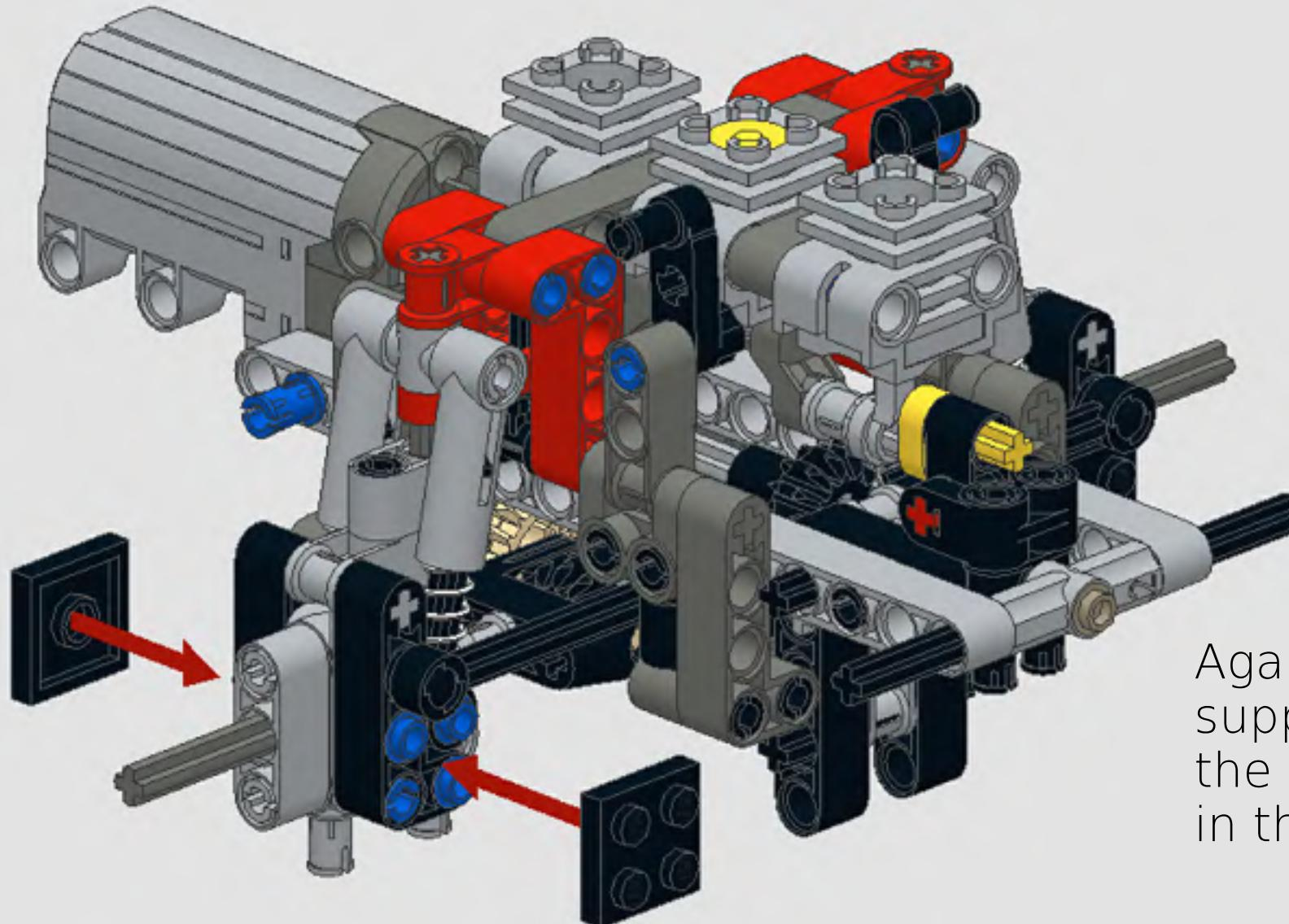
Again, make sure the supporting axle and the driving axle are in the right place.
