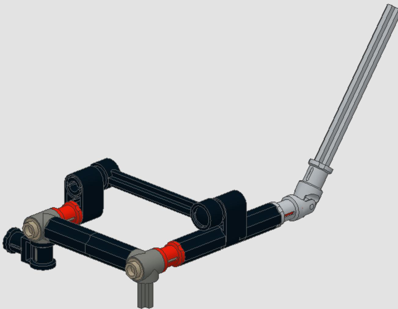
This might sound weird but is actually very important. You have to make sure that the universal joint is in the exact position as in this picture. If it would be rotated by 45 degrees (meaning that the little axle pointed out below is vertical instead of horizontal), much less movement gets transferred through the joint. Try it yourself!
