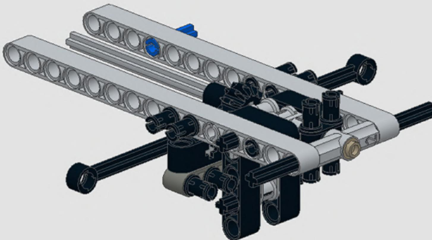
Make sure the gear rack is perfectly centered, and carefully position the gear so that the axle running through it is centered as well.
