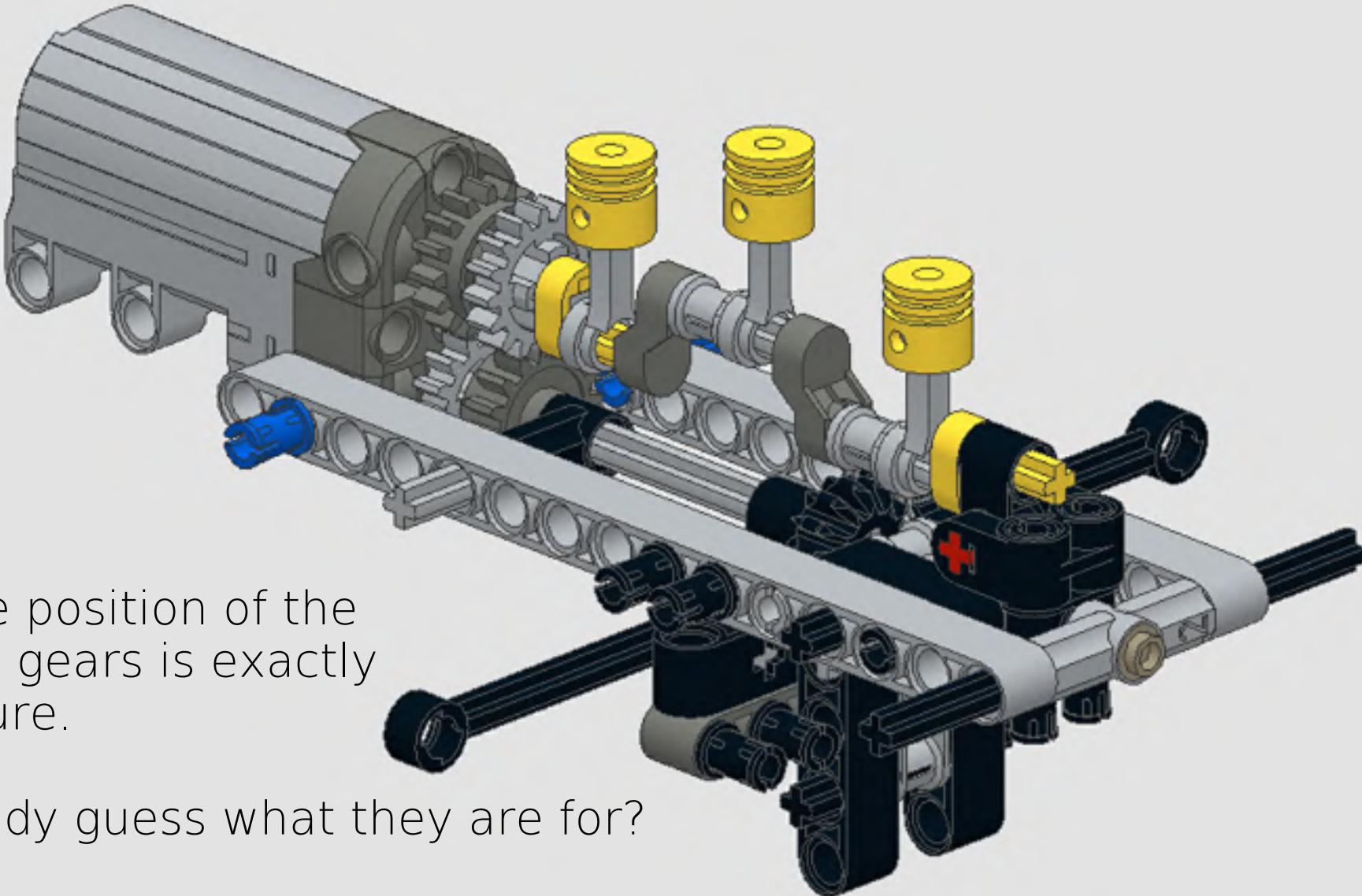
Make sure the position of the light and dark gears is exactly as in the picture.
