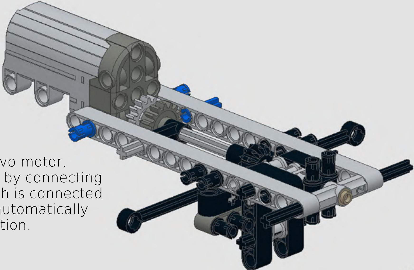
Before mounting the servo motor, make sure it is centered by connecting it to an IR receiver (which is connected to a batterybox). It will automatically rotate to the center position.
