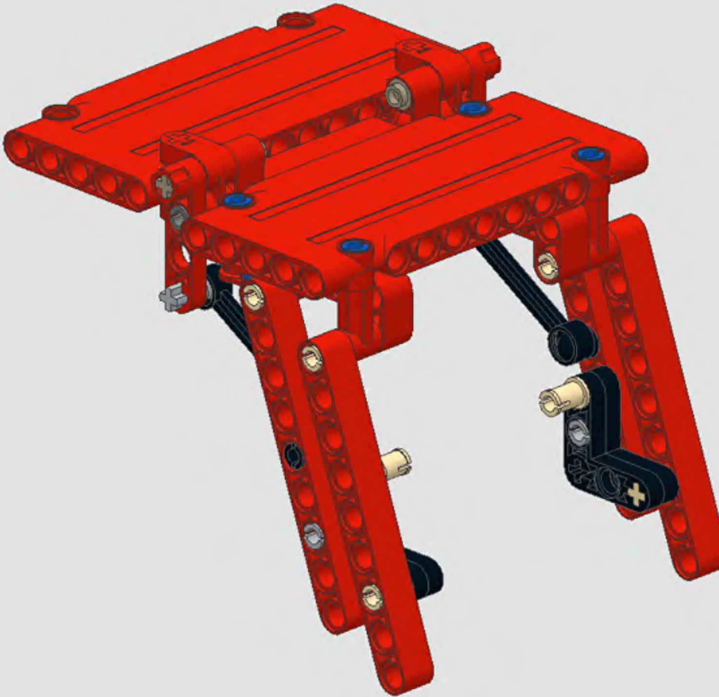
The roof has to be attached to the grey pins that are sticking out.
