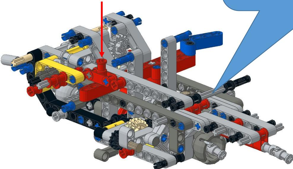
This 5L axle here is not necessary, and you should in fact *not install it!* You should also flip the long friction axles w/bush (black) to have the bush point *outwards*.
