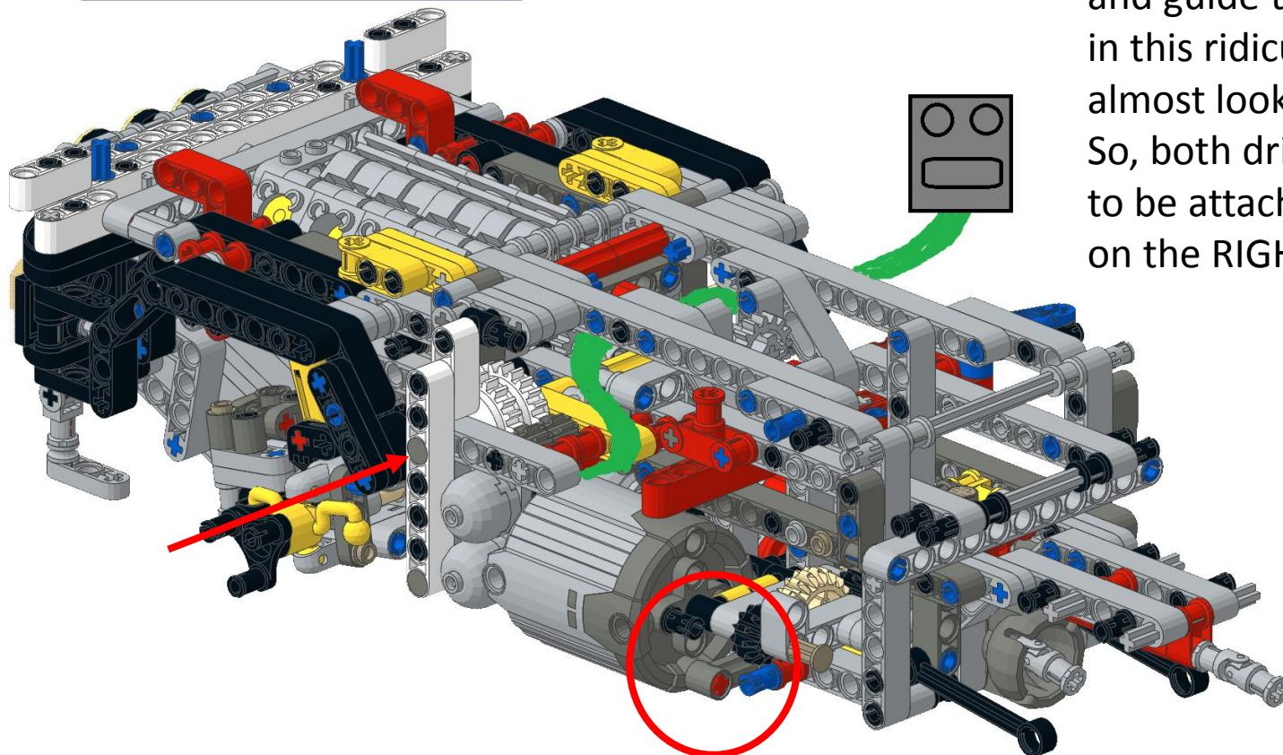
OK, so place the white assembly where indicated, push the XL motor in from the left so it attaches to the exposed pins, and guide the wire like indicated in this ridiculous picture. Look, it almost looks like a happy face! So, both drive motors are going to be attached to an IR Receiver on the **RIGHT** side of the truck.
