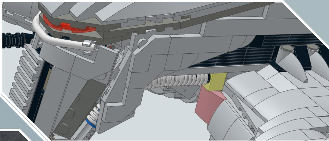
**NOTE:** you will need to remove the 2x2 curved slopes (highlighted in red here), to insert the 1x1 Technic brick with hole on the loose end of the ribbed hose (highlighted in yellow).
