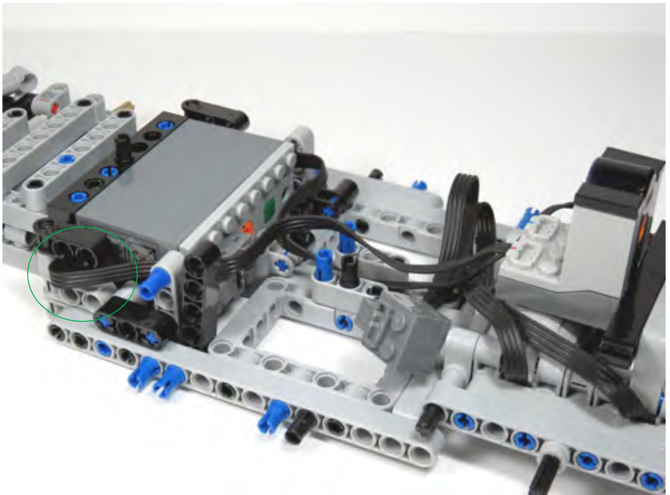
IR receiver cable runs up through the centre, then to circled area, then to battery
